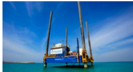
Horizon 27 Self Elevating Platform. Operating in the Middle East and Indian Ocean
