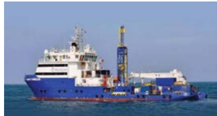
Quest Horizon 65m DP2 Geotechnical Site Investigation Vessel. Operating in the Middle East and Indian Ocean
